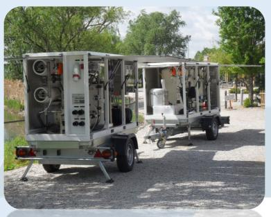
This system offers a modular solution for the production of drinking water from brackish water sources.
