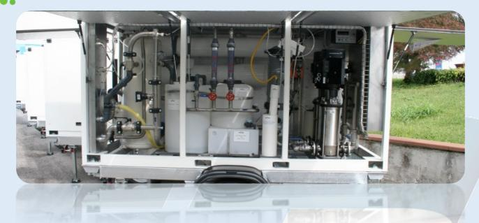
The **IT-BW-CL (Chlorine)** water treatment unit is designed to produce drinking water from brackish water with TDS up to 6000 ppm (it will not treat sea water) and is ideal for treating water in remote areas with limited water resources.
