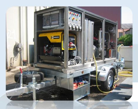
The **IT-BW-SA (Stand Alone)** water treatment unit is designed to produce drinking water from limpid brackish water with TDS up to 2000 ppm (it will not treat sea water) and is ideal for treating water in remote areas with limited water resources.
