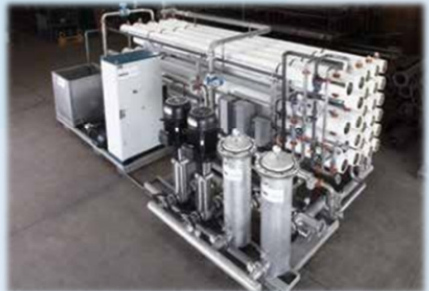
Reverse osmosis plant Q = 2500 m 3 /day.
