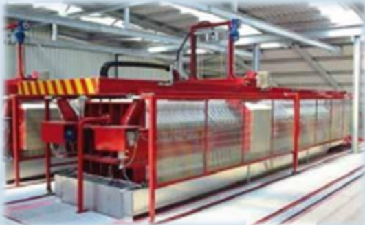
Filter press for sludge dehydration.
